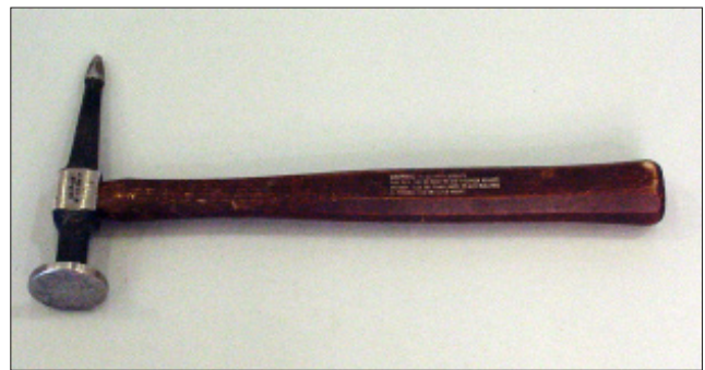
I-5 A pick hammer may be used for metal finishing.
