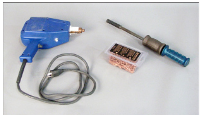
M-3 A kit may be available that includes the stud gun, pins, and slidehammer.
