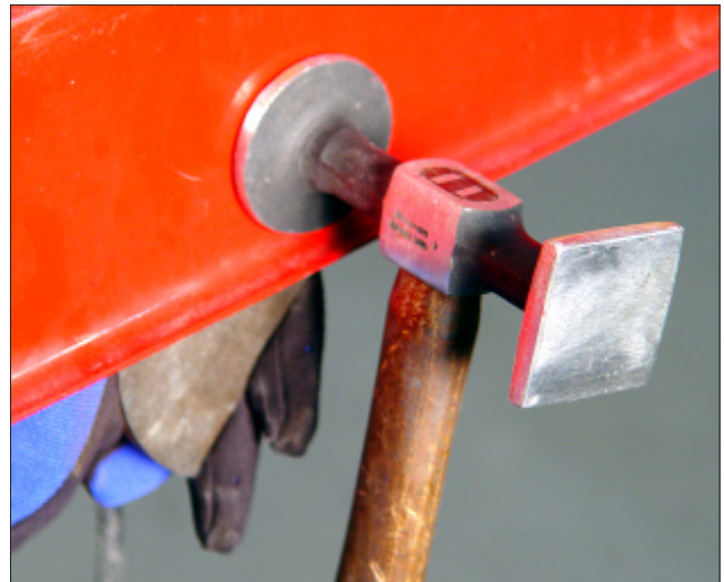
F-4 Hammer force affects how the hammer-on-dolly technique removes the damage.
