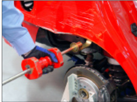
N-2 A flat hook tip used with a slidehammer can be used to gain access at the edge of a panel.
