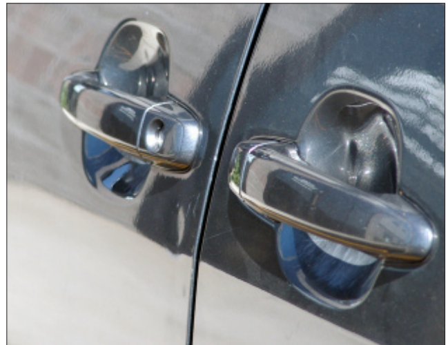
C-12 The durability of a repair near a door handle may be compromised by stress and wear to this area of the panel.
