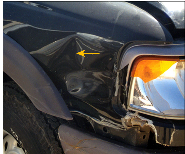
A-14 The concave center of this damage is the collapsed roll buckle area.
