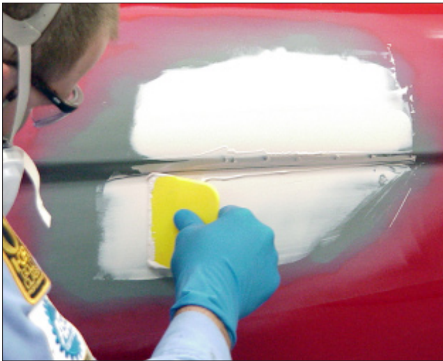
E-6 Do not apply body filler to areas that have not been properly sanded.
