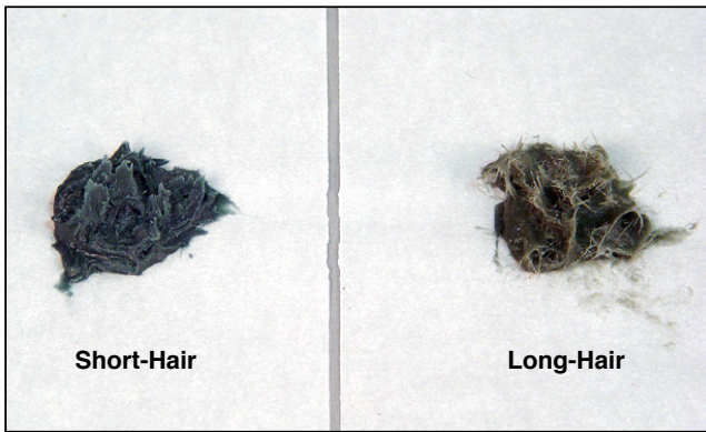
B-8 A long-hair fiberglass filler may be more difficult to smoothly apply compared to a short-hair type.
