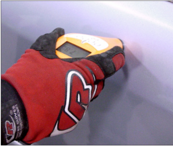
C-7 A film thickness gauge should not damage the finish.
