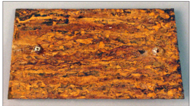
A-6 A corroded piece of metal is weaker than a piece that is not corroded.
