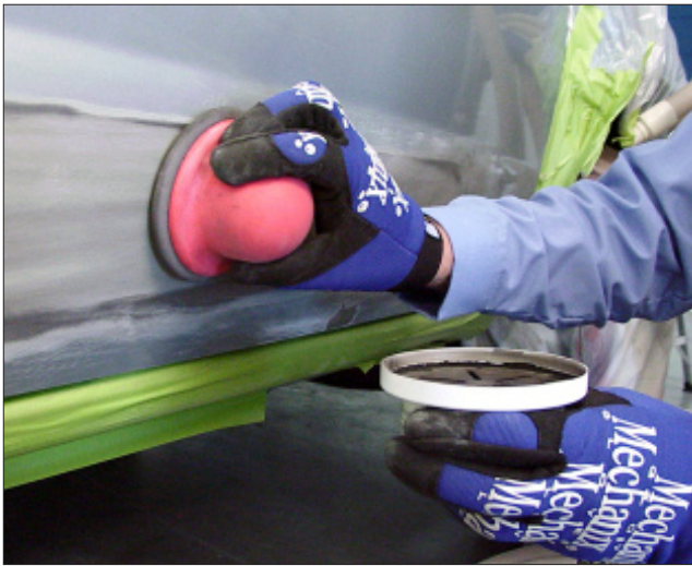
H-5 Guide coat can be used to help identify the high and low spots when sanding body filler.
