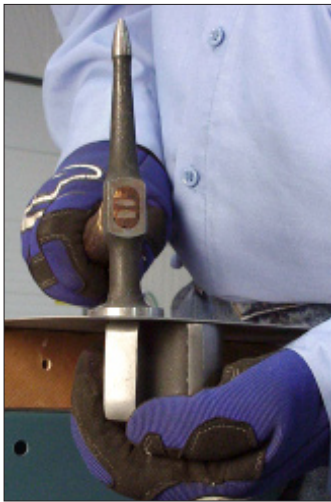
F-3 When using the hammer-on-dolly technique, the tools are directly on top of each other.
