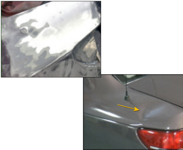
I-1 The repair to this quarter panel will not require the use of body filler.
