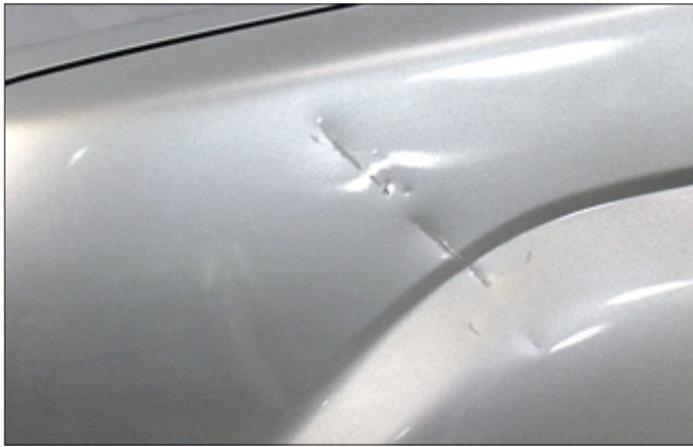
B-1 Because this damage extends into multiple contours of the panel, a combination of repair methods will be used.
