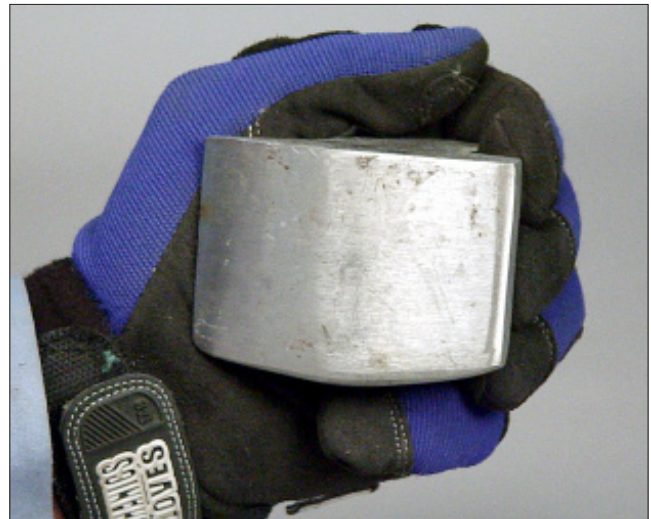
E-4 If this side of the dolly was used like a hammer, it would cover a larger surface area than the face of a hammer.
