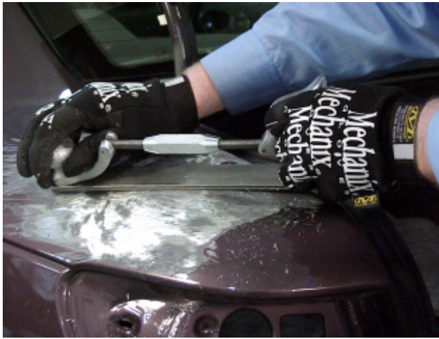
I-12 Even pressure on the body file must be used to accurately identify high and low spots.
