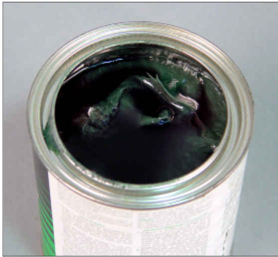
D-2 The solid and liquid have separated in this can of body filler.
