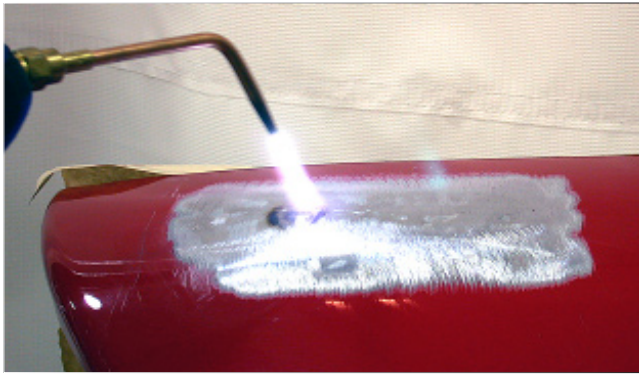
L-4 Typically the sharpest area of a crease is at one end and is gradually worked to the other end.
