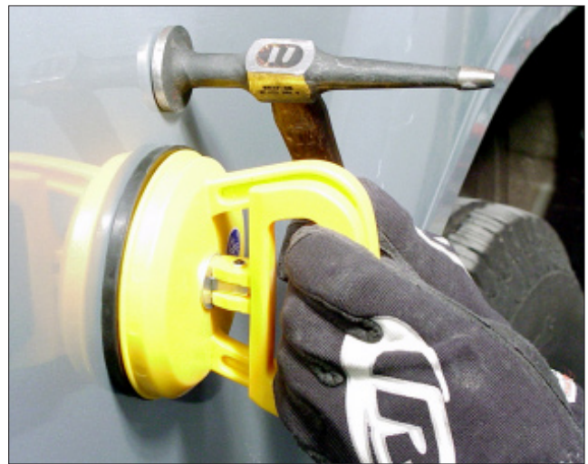
N-1 After using suction to repair damage, refinishing may not be required.
