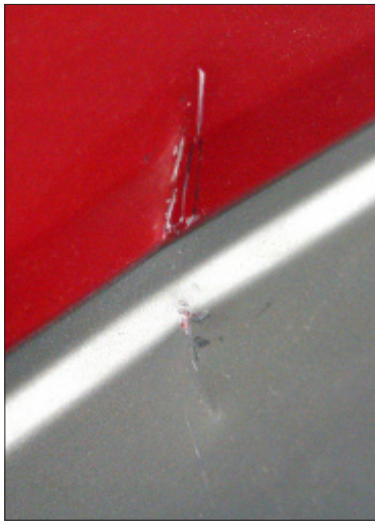
H-4 A sharp force was used to create this type of damage to a feature line.
