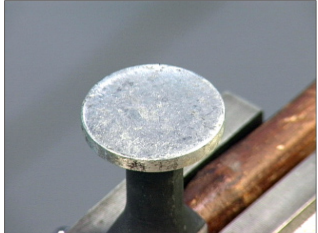
D-7 The marks on the face of this hammer may imprint the sheet metal causing additional damage.
