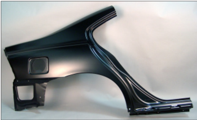
C-3 This quarter panel was made using cold-rolled sheet metal.
