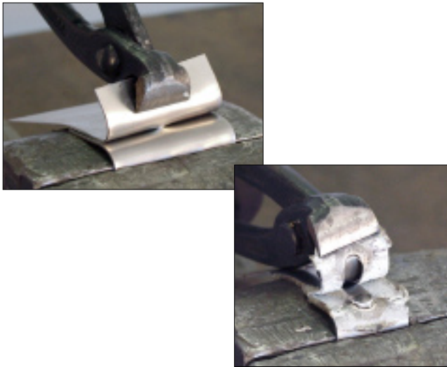
A-16 Tension is used to try to pull this weld until it peels apart.
