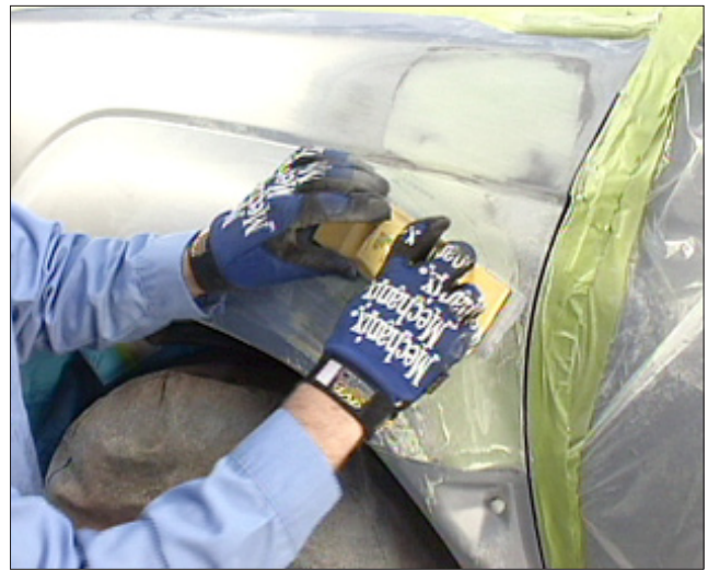
B-4 Separate contours within a panel may allow the body filler to be sanded in separate stages.
