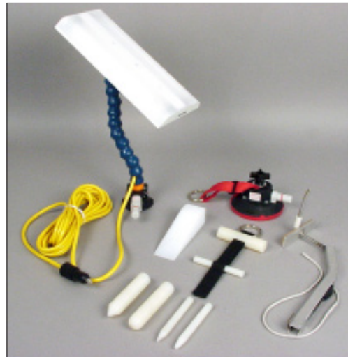
C-5 PDR technicians sometimes may make their own accessories to fit their individual needs and preferences.
