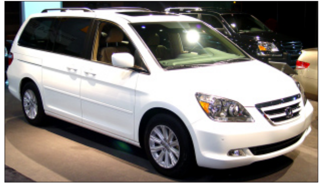
C-11 The body lines on this vehicle's doors act as reinforcements that may affect the ability to remove damage.
