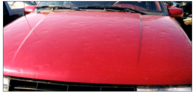
C-3 The number of dents in this hood is excessive.
