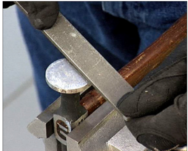
D-13 This technician is using a fine tooth file to remove the surface imperfections from the face of this body hammer.
