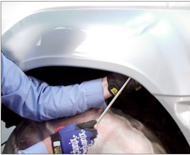
I-8 A fulcrum point is required to raise the low spot.
