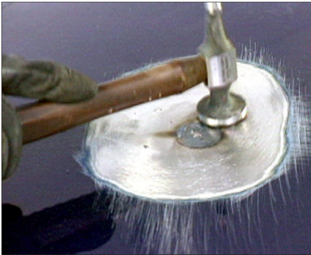
K-5 Tap lightly when hammering during heat shrinking to prevent distorting the softened metal.
