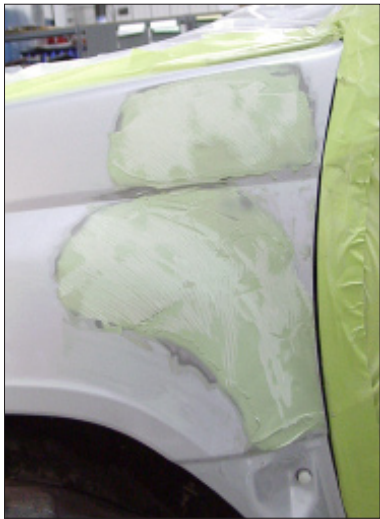
H-3 The highest areas of the body filler will be sanded first.
