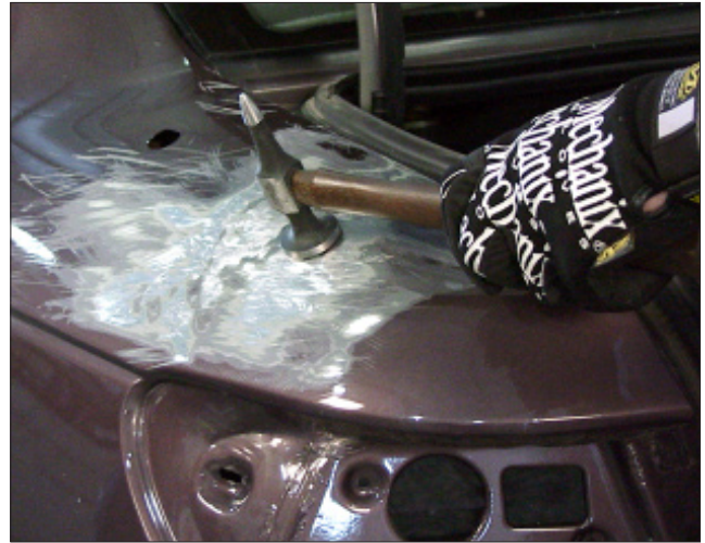
H-11 A finishing body hammer is used to straighten the panel to the proper contour.
