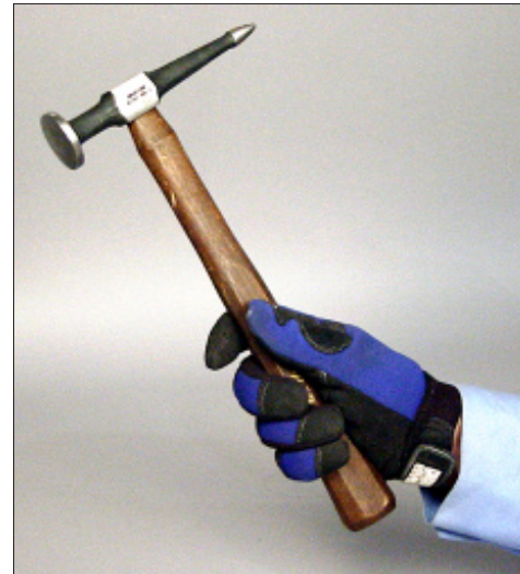
D-9 This is an example of how to properly hold a body hammer.
