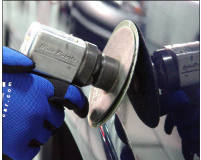
C-5 The face of the grinding disc should not be held flat to the surface of the panel.
