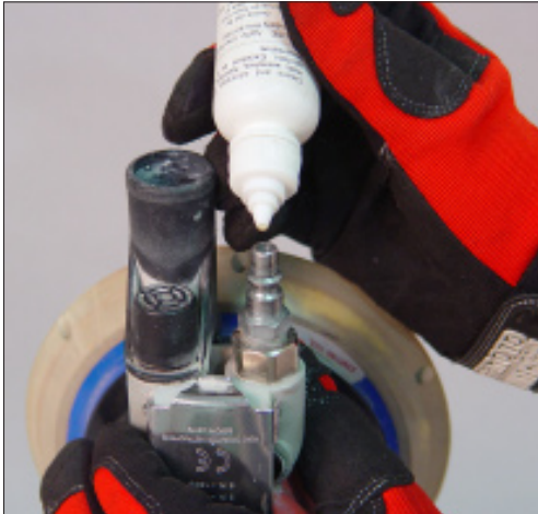
F-5 Pneumatic tools are lubricated using a specific oil.
