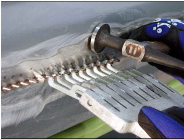
M-10 A hand puller may be used with wiggly wire to apply pressure similar to a slidehammer.
