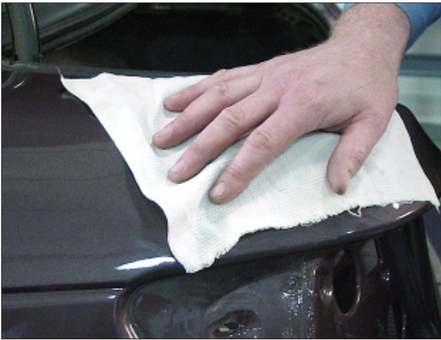
B-3 The high and low spots are identified before the damage removal begins.
