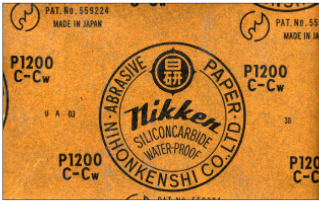
G-10 This piece of sandpaper is made using silicon carbide as the abrasive.
