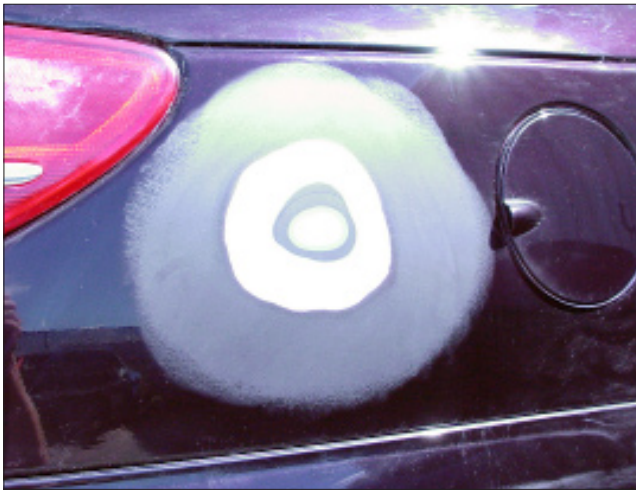
C-8 The paint is sanded so that the edge of each coat is visible.
