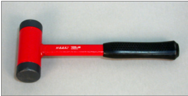
G-6 A dead blow hammer may have an interchangeable head according to the repair.
