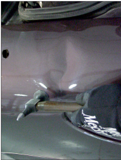
A-6 Striking a panel with a hammer will straighten areas adjacent to a buckle because of spring-back.
