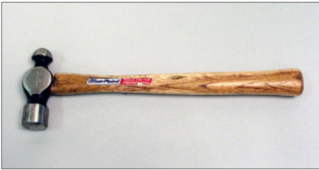
G-5 The pick end of the ball peen hammer has a larger surface area than a body hammer.
