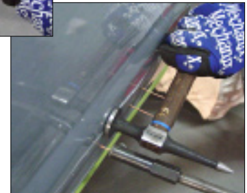
M-5 While a slidehammer is applying pressure to the pin, a hammer is used to relieve the tension on the panel.
