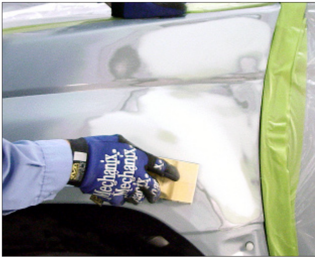
B-5 Along with the contour of the panel, the feature lines must also be sanded to match the rest of the panel.
