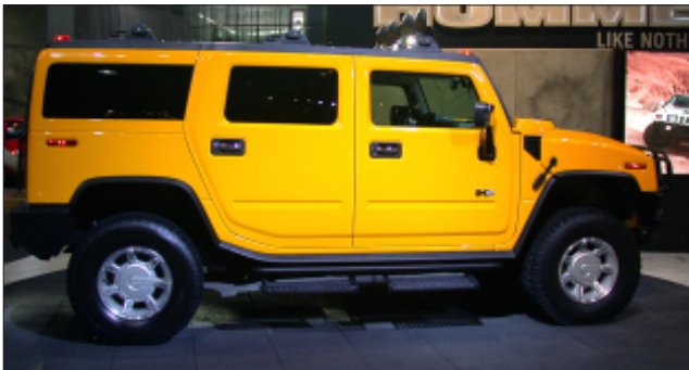
D-2 The 2004 Hummer H2 has flat areas on the doors and quarter panels.
