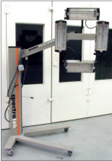
E-1 An infrared lamp may be used to warm cold metal parts.
