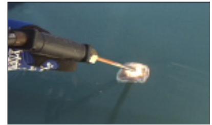
K-4 Heat shrinking can be done by inducing heat through electricity.
