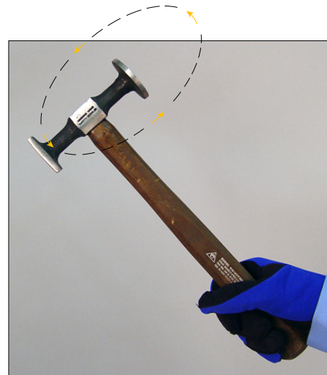
D-11 This is the type of circular motion that should be followed when using a body hammer.
