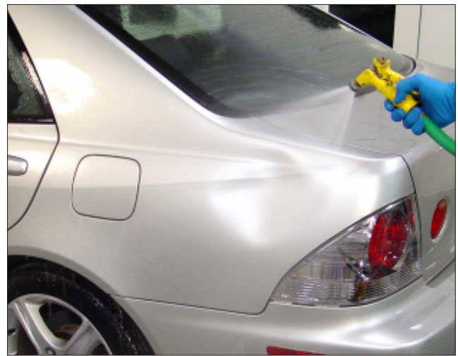
H-8 It is important that the repair area is clean before beginning repairs to prevent contamination and addition damage.
