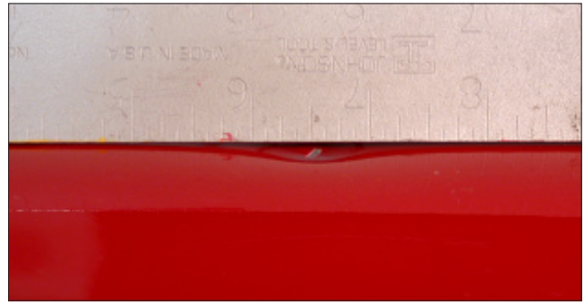
B-4 A metal ruler is an example of a straightedge that can be used to identify a low spot.
