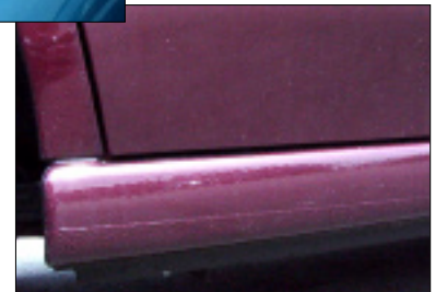
E-7 Repairs to a hood near the hinge or on a rocker panel may fail over time.
