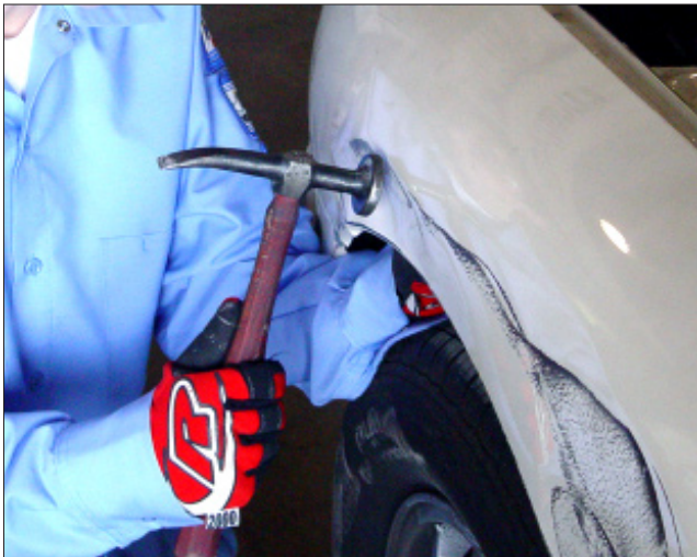
H-10 The technician is using the hammer-off-dolly technique for intermediate straightening.
