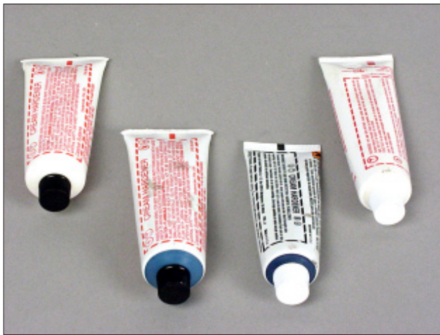
D-4 The color of the hardener is different than the body filler that it will be mixed with.
