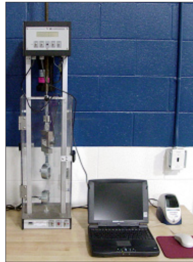
A-14 A tensile-strength machine can be used to determine the yield strength of a material.
