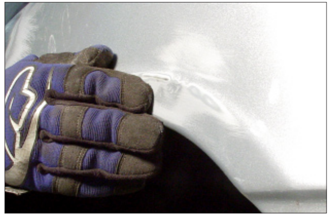
B-6 Feeling for high and low spots is an acquired technique that can be used throughout the repair process.
