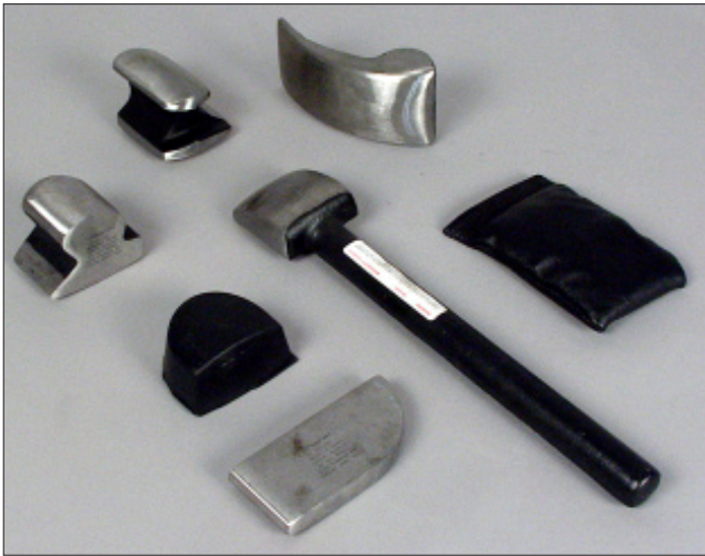
E-1 Different types and shapes of dollies are used to repair damage.
