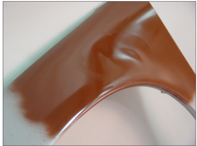
J-11 Applying heat may result in warping the panel.
