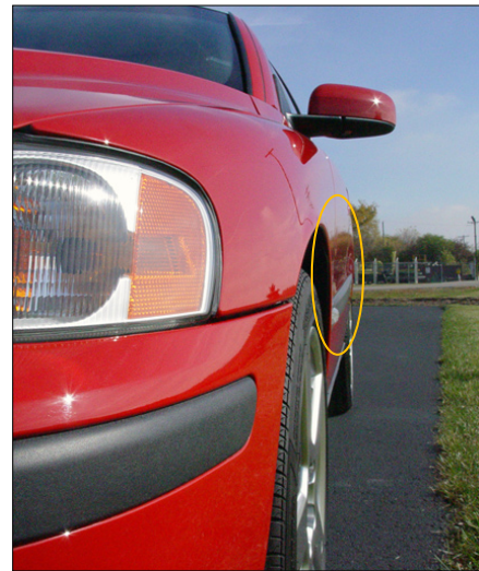
D-7 The low crown area of this door almost looks flat.
