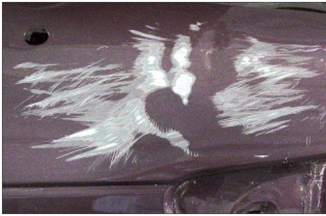
B-7 The bare metal areas are the highest spots and the areas with paint are the lowest spots.
