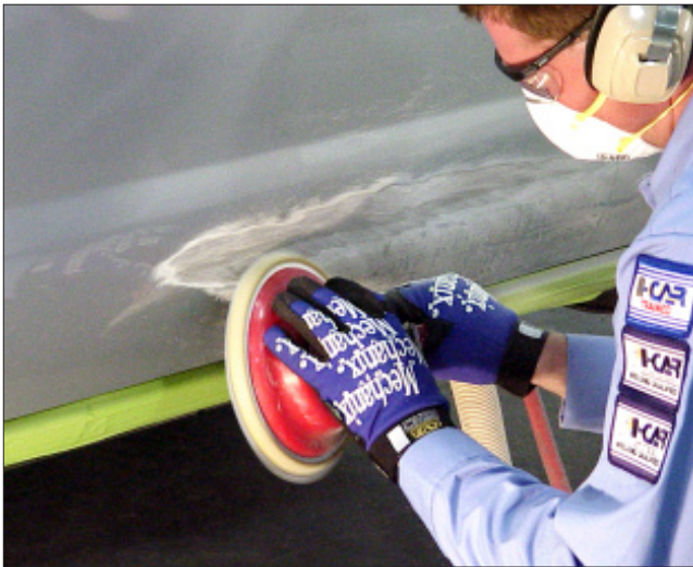
C-2 Body filler should not be applied to a smooth painted surface.
