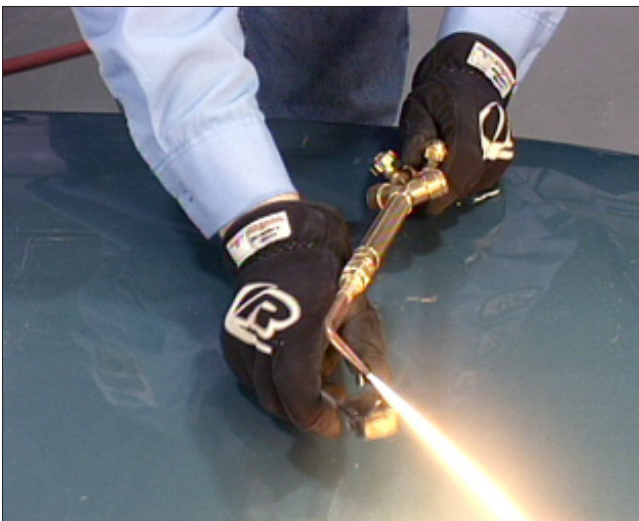
J-14 Minimal temperature is required to shrink thin metal.
