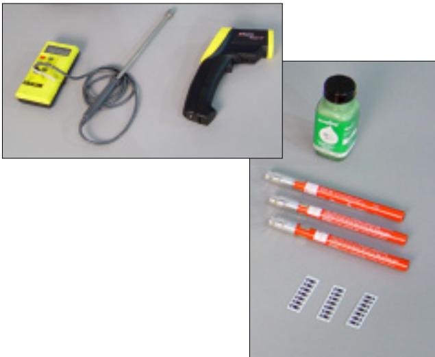
J-7 Temperature indicators are used to monitor the heat affect area.
