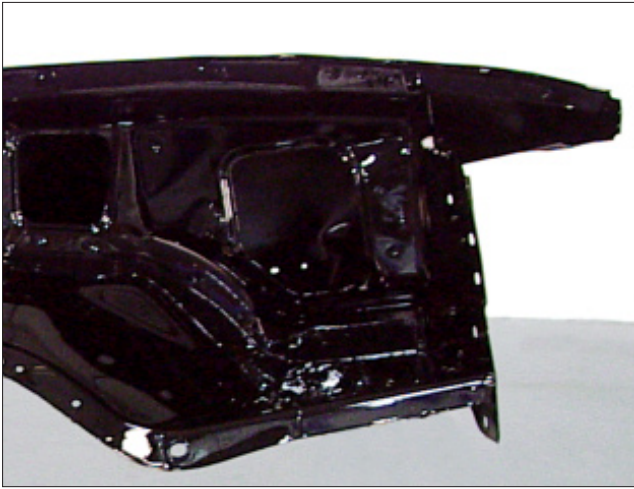
C-9 The part design of this fender restricts access to the damage from the backside.
