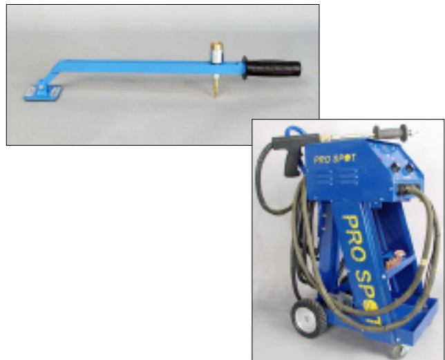
M-7 Leverage bars and dent removal tools may be dedicated just for dent removal.
