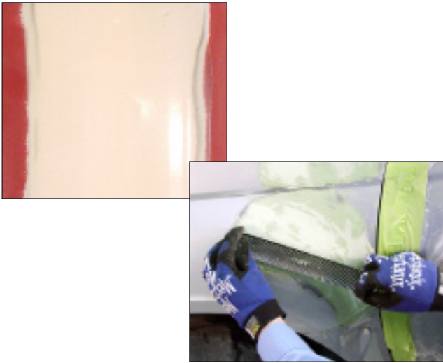
B-3 A cheese grater may be used to remove the shiny paraffin produced by some body fillers
