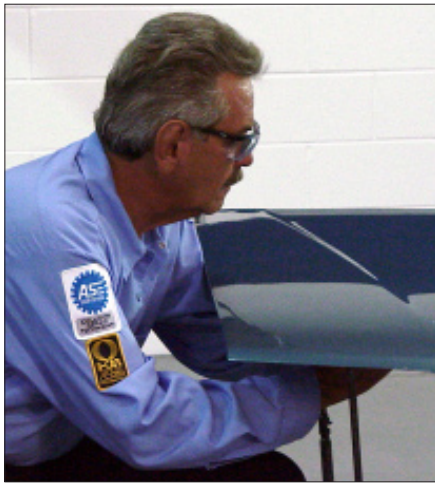
C-2 PDR technicians use lighting to monitor the dent removal process.
