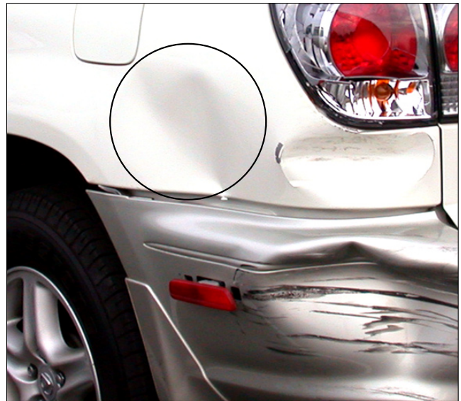
A-16 The direct damage below the rear tail lamp has caused this area of the quarter panel to be displaced.
