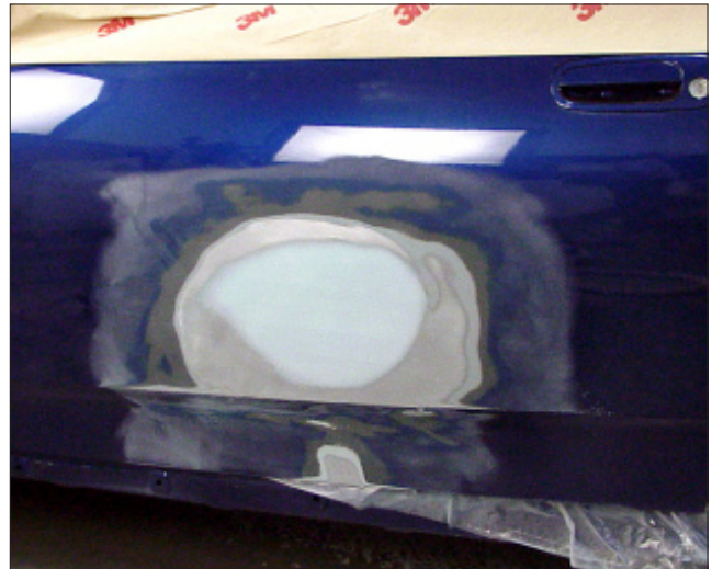
H-8 The contour of the panel has been restored.
