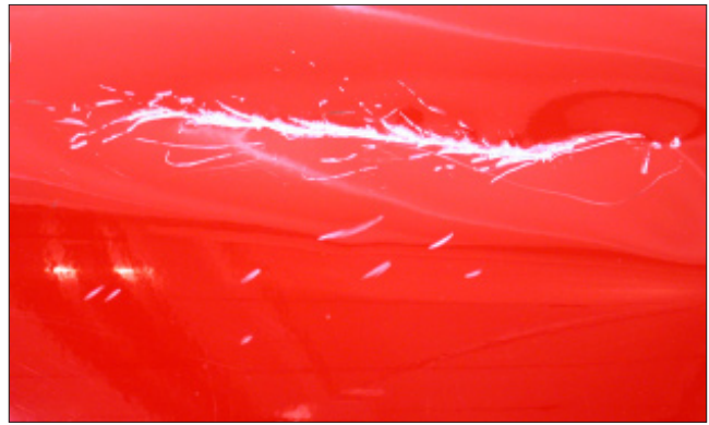
L-2 A sharp crease will stretch the metal.
