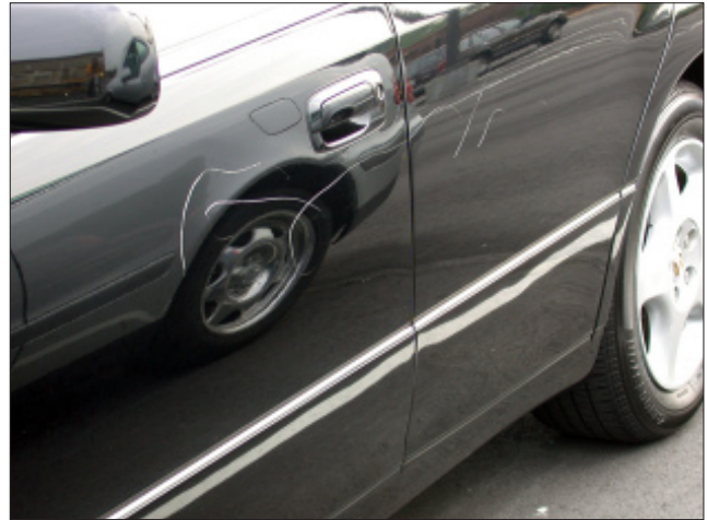
A-3 A sharp object, such as a key, was used to vandalize the finish on this vehicle.
