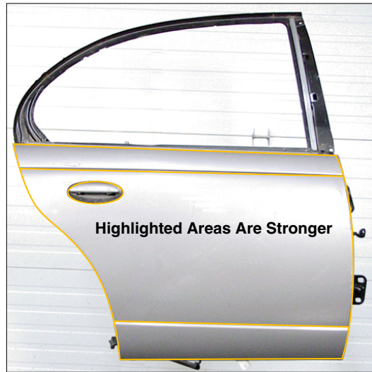
H-1 Some areas of a panel are stronger by vehicle maker design.
