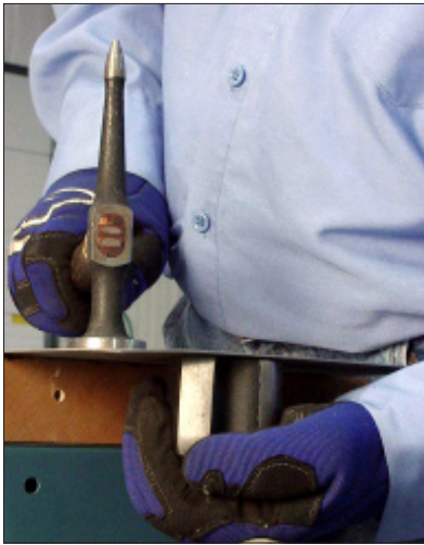
F-7 When using the hammer-off-dolly technique, the tools should not touch each other through the panel.
