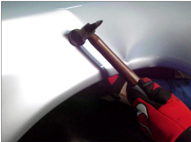
D-10 The amount of hammering force required may vary from dent to dent.
