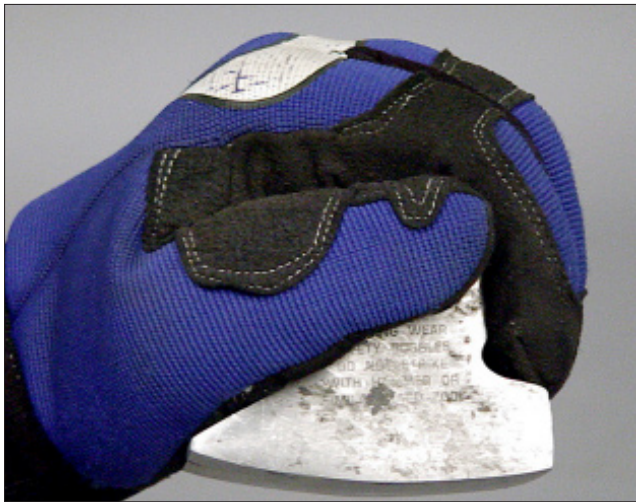
E-3 This is an example of how to properly hold a dolly.
