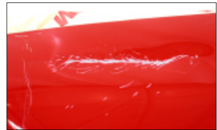
L-3 A dolly can be used on the backside of the panel to raise the crease above the surface.
