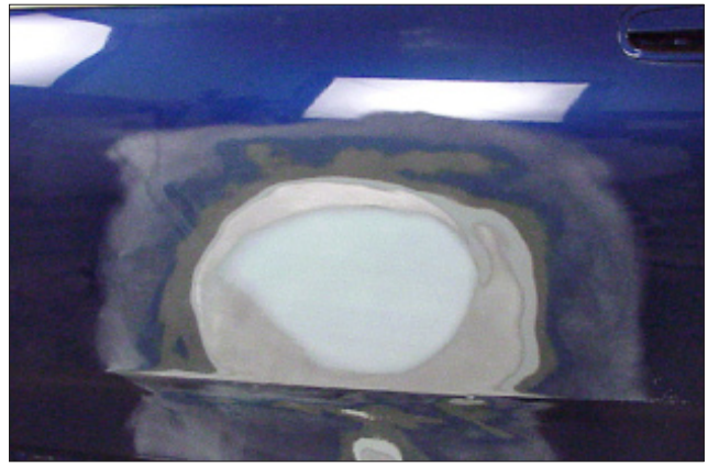
D-9 Body filler shrinks when it has cured.
