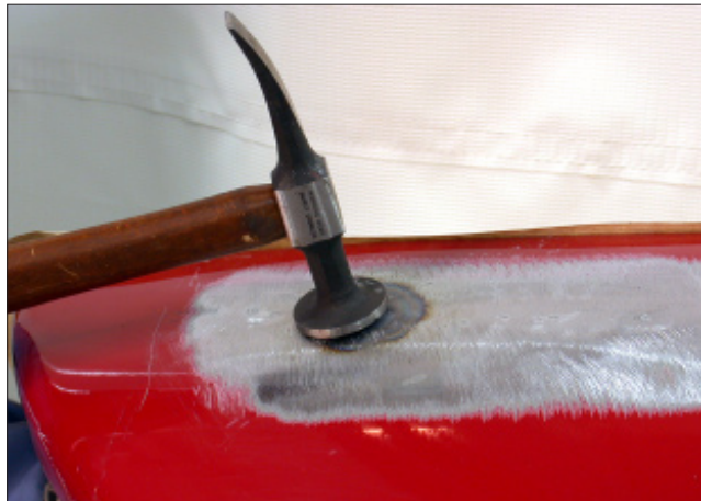
L-5 The hammer-on-dolly technique is used to shrink a crease.
