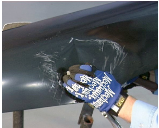
F-2 The dolly may be held on the front side of the panel while a hammer is used to strike the backside.
