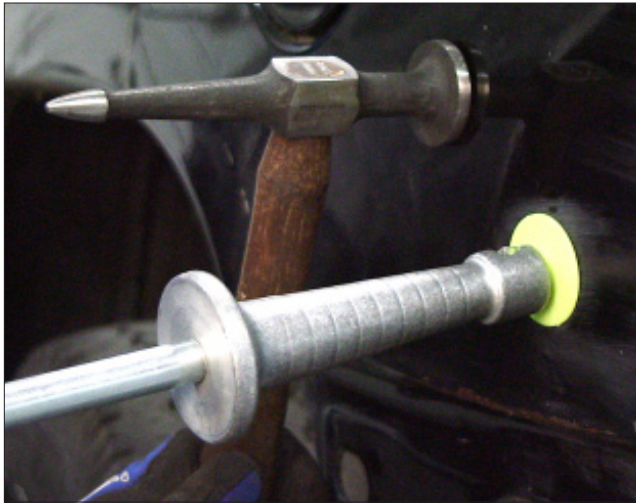
N-4 This slidehammer slips over the collar of the adhesive disc.
