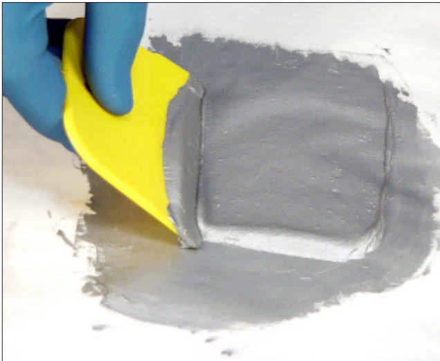
B-10 Compared to the other types of body filler, it is not as easy to tell when aluminum body filler and hardener are mixed thoroughly.
