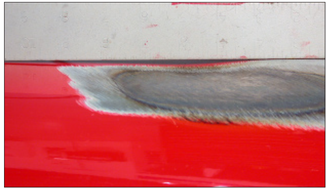
K-8 Notice the gap between the straightedge and the panel indicating overshrinking.
