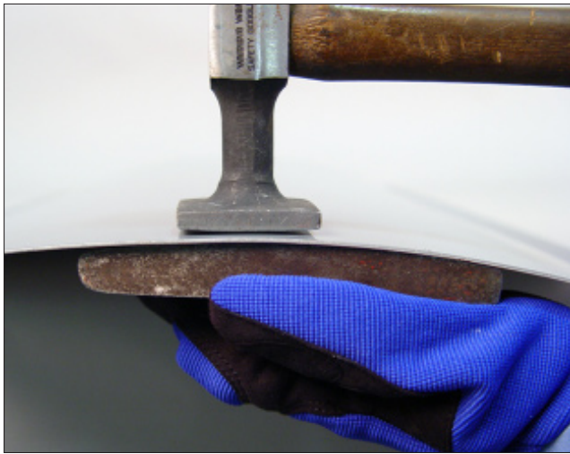
F-5 When the hammer strikes the panel, the location of the dolly is critical.
