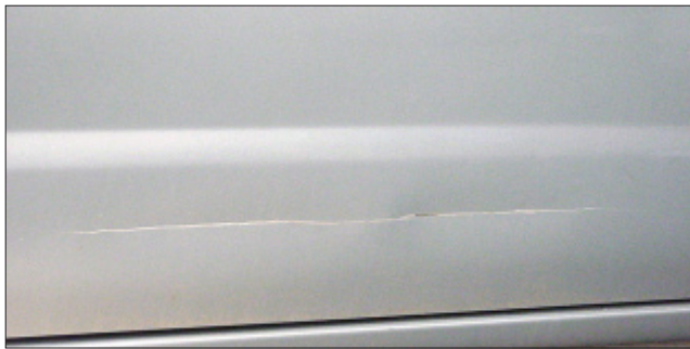
L-1 The bottom of this door has a long crease in it.
