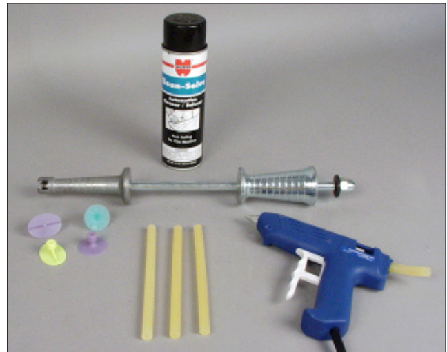
N-3 Adhesive dent removal kits are available that include equipment required for repair.
