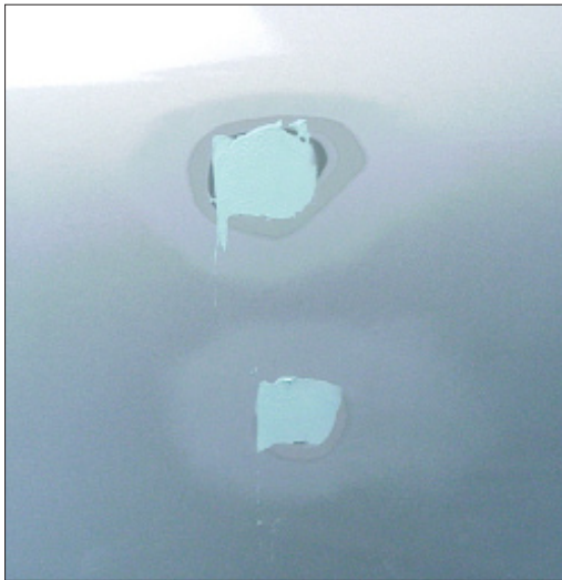
B-14 Thin coats of polyester glazing putty should be used.
