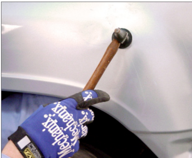
H-5 A hammer and dolly can be used to remove damage without the use of heat.
