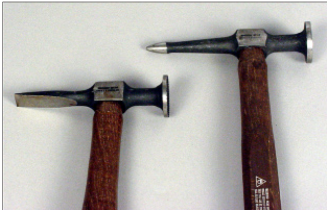
D-6 The head of the hammer is used to strike the panel.
