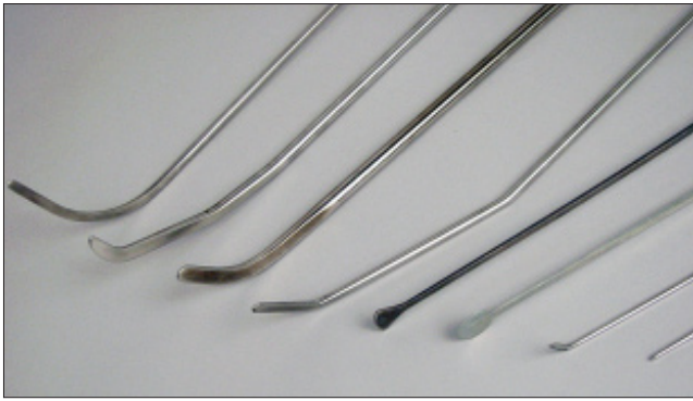
I-6 Many different pick tips have been designed to access and remove damage.
