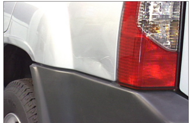
C-6 The damage to this quarter panel is not easily accessed from the backside.
