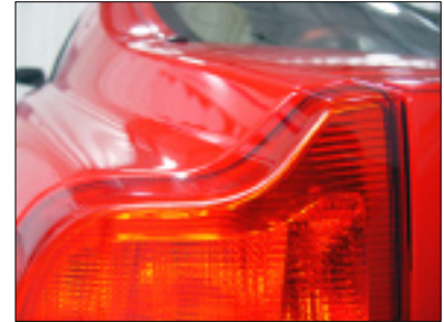
D-9 The reverse crowned area is concave instead of convex.
