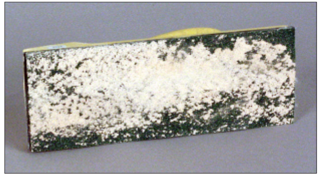
D-12 This sandpaper was used on body filler that was not completely cured.
