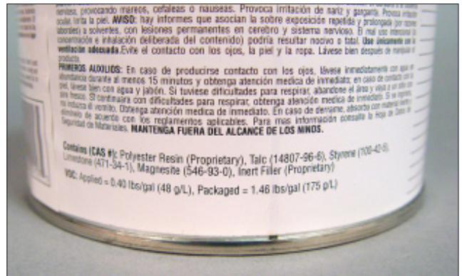
B-5 Talc is the basic pigment in many of today's body fillers, but it is not the only pigment.
